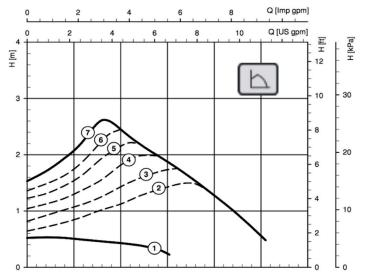
So how do you set such a pump? The pump needs to be strong enough to provide heat for the whole house, and therefore you should set it to reach maximum head when all valves are open. If you know your maximum design flow, you can pick that point out of the pump diagram. If not, you open all the thermostats in the house fully (assuming hydraulic balancing has been done), and then increase the power setting slowly until you see that the head pressure is not increasing anymore.
