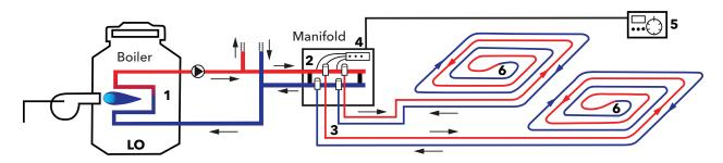
Therefore, the pump should supply the individual loops of the underfloor heating system with the same head pressure regardless of how many rooms are being heated.
