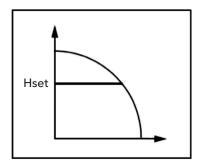
The setting of such a pump is comparatively easy. The underfloor heating manufacturer will have specified the correct differential pressure for the individual loops, and the pump just needs to be set to this value. If necessary, adjustments can be made to counter noise or insufficient heating.
